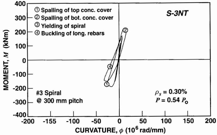
Fig. 4. Moment-Curvature Response of Specimen S-3NT.
