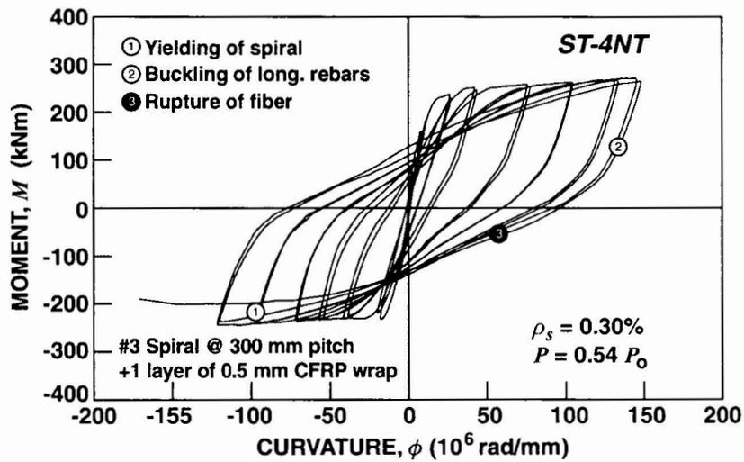
Fig. 8. Moment-Curvature Response of Specimen ST-4NT.
