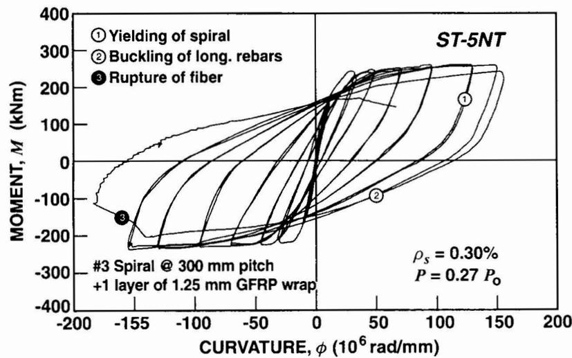
Fig. 9. Moment-Curvature Response of Specimen ST-5NT.
