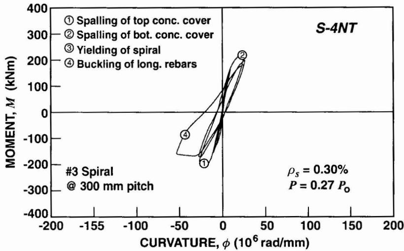
Fig. 5. Moment-Curvature Response of Specimen S-4NT.
