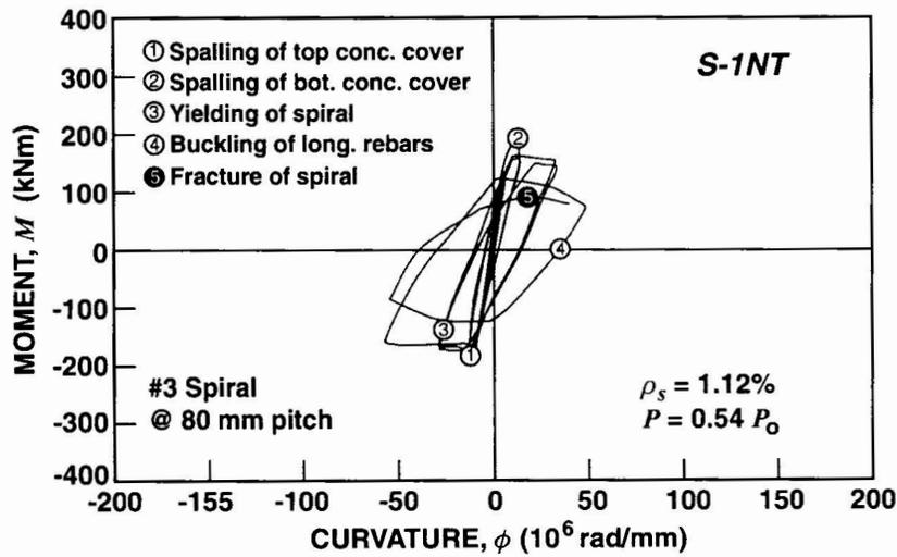
Fig. 2. Moment-Curvature Response of Specimen S-1NT.
