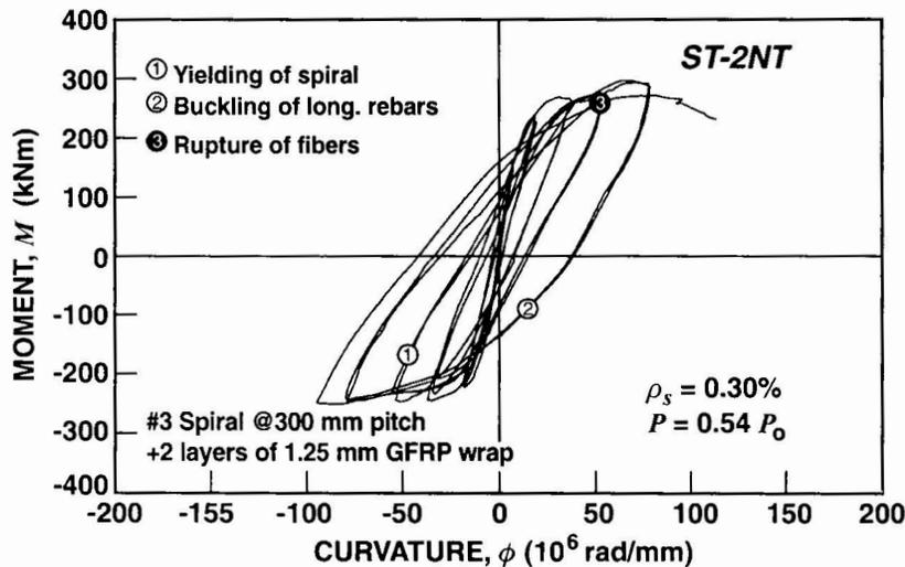
Fig. 6. Moment-Curvature Response of Specimen ST-2NT.
