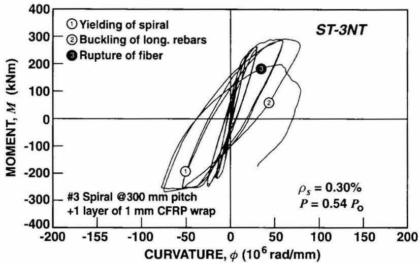
Fig. 7. Moment-Curvature Response of Specimen ST-3NT.
