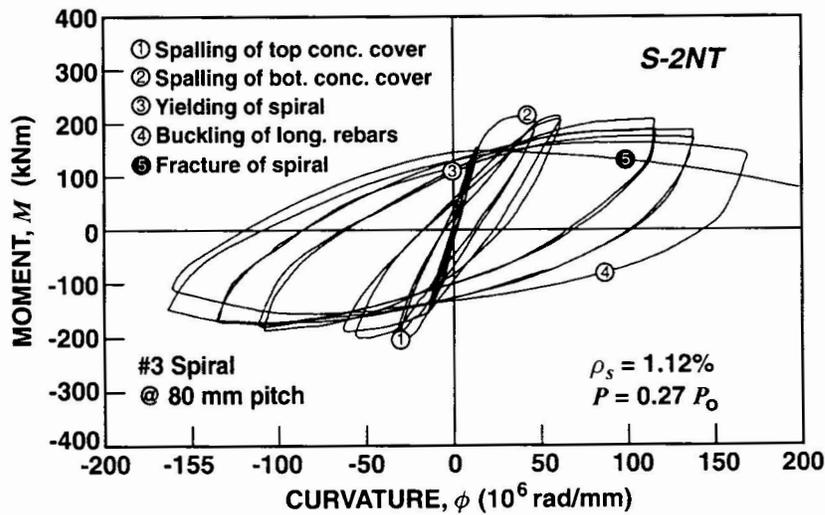
Fig. 3. Moment-Curvature Response of Specimen S-2NT.
